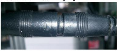
6. 將溫控攪拌器電源連接到控制器。 Plug the connection to Temperature and Stir Speed Control Panel.
