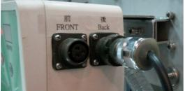
● 請將前側接頭拔除,請旋轉後再拔除。Disconnect the plug indicated as FRONT.
