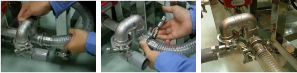
連接排水管即可完成 And connect the water drain pipe. The installation is done.
