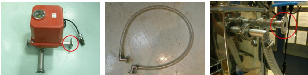
冷卻水套進水管 water into chilling water tank installation.
