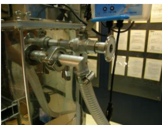
冷卻水套進水管 water into chilling water tank installation.
