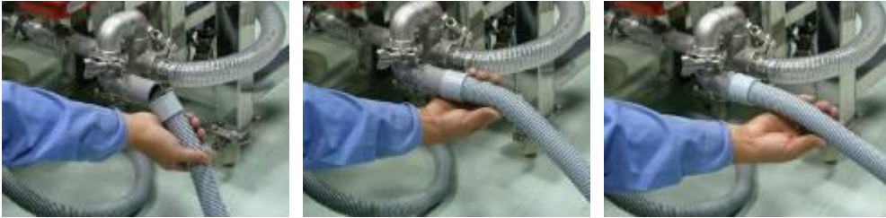
連接排水管即可完成 And connect the water drain pipe. The installation is done.
