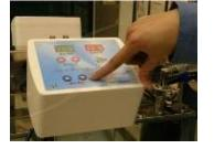
Main power button (this button is designed for anti-water)
