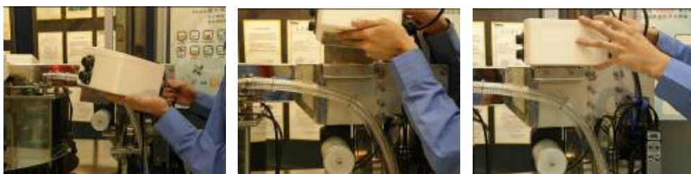
以六角板手固定控制器 Use no. 6 ratcheting wrench to fasten the control system box.
